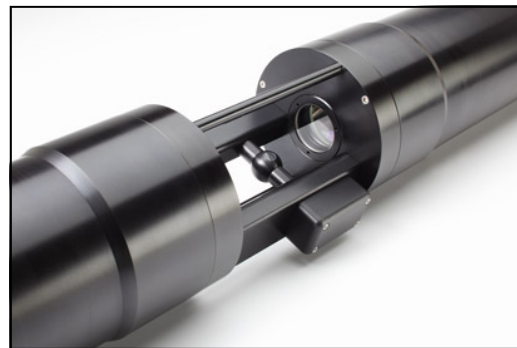
Detail of the LISST-VSF optics path, showing the receive optics and the Roving Eyeball
